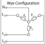
For Delta configuration, a three-phase wire and a ground are supplied. For a Wye configuration, a three-phase wire, a neutral, and a ground are supplied. The configuration and voltage are declared on the unit name plate on the enclosure front type plate.
