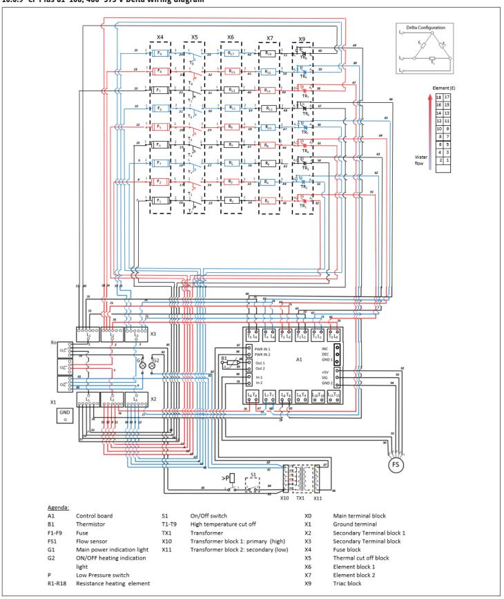
10.6.10 CF Plus 120-144, 480 V Delta wiring diagram
